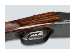
To adjust the trigger position, loosen the trigger position lock screw (which faces towards the muzzle), using the 1.3 mm hex wrench provided (see illus. No.8). The rear opening does not contain anything. Slide the trigger blade to the desired position and gently retighten the trigger position lock screw.
