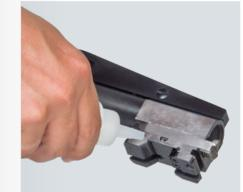
Gun Glide is a high quality grease that protects guns from heavy wear. Use it as described above on the heavy wear areas of the KX-6 Special and other break-open guns: the barrel pivot point, and the area just behind the back of the barrel lug; the face of the ejector, where it meets the face of the breech; and the rear surface of the forend iron where it pivots on the receiver.
